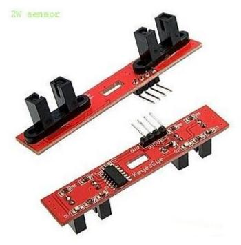
The module is intelligent car speed measurement module! It adopts groove—type photoelectric correlation and can be triggered once the non-transparent object passes through the groove (used in conjunction with car encoder sold in our shop)! It is equipped with schmitt trigger to eliminate vibrating pulse. It can be applied to distance measurement as well as rotate speed measurement of cars! and our car encoder)!
