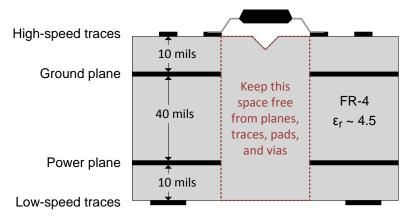
Figure 34. Recommended Layer Stack
