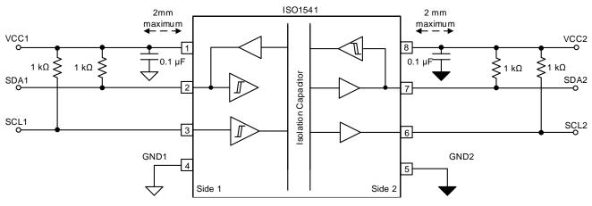
Figure 32. Typical ISO1541 Circuit Hookup
