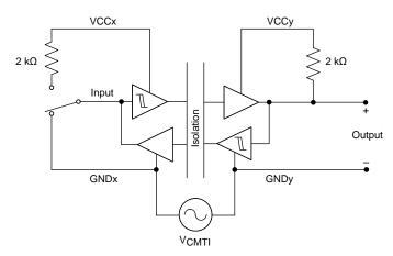
Figure 21. Common-Mode Transient Immunity Test Circuit
