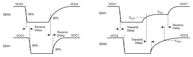
Figure 26. SDA Channel Timing in Receive and Transmit Directions
