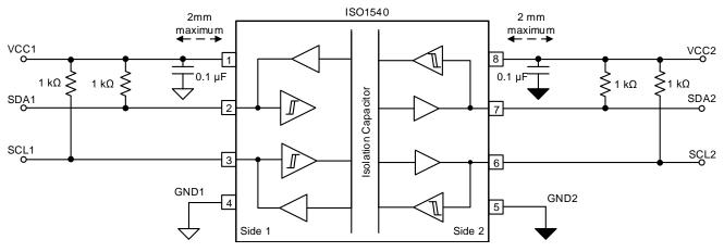
Figure 31. Typical ISO1540 Circuit Hookup
