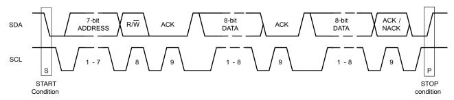
Figure 28. Timing Diagram of a Complete Data Transfer
