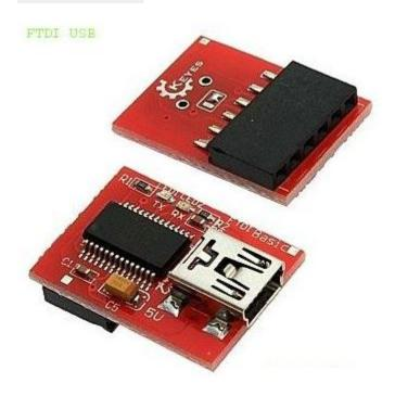
This module provides users with alternatives of module power supply. Three solder joints in the diagram below, the bottom one is for 5V, upper one for 3.3 V. Users can choose power supply according to corresponding USB's power supply voltage. Just weld it on with soldering iron. USB to serial port can be used together with Arduino mini. Plug Arduino mini to corresponding pins of the convert module, you can then upload arduino program to Arduino mini.
