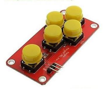
Arduino electronic building blocks AD the rid\_device\_info\_keyboard analog Keyboard module Arduino special module, port compatible sensor analog Keyboard extension board, 5 buttons only takes up an analog port, save resources, analog acquisition, press a different button different voltage output, high quality omron key, sensitive and durable, suitable for the arduino platform, compatible with the arduino sensor interface
